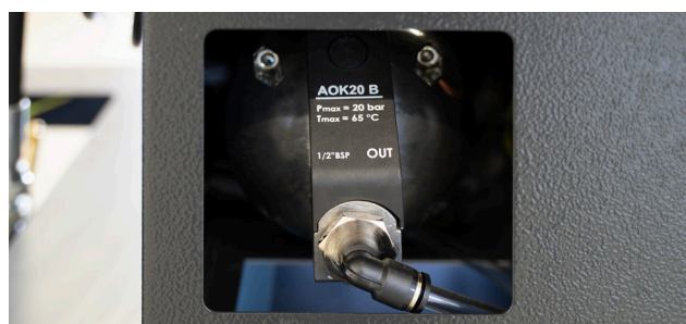
Lossless float-based condensate drain
